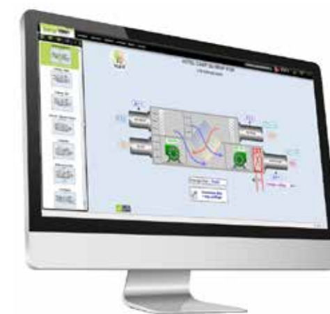
↑ EV CTA : Supervision GTB Energy Vision de Delta Dore.
